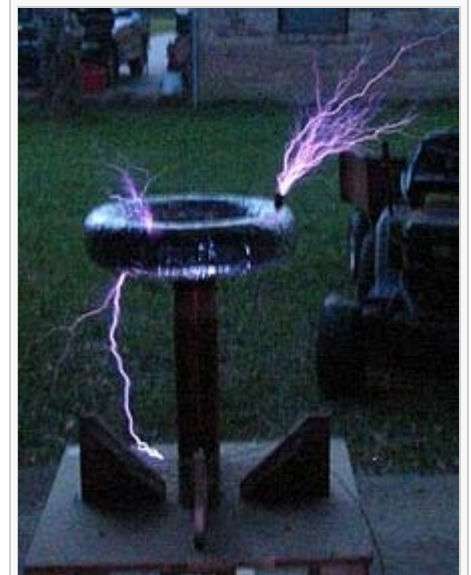
A small, later-type " Tesla coil " in operation. The output is giving 17-inch sparks. The diameter of the secondary is three inches. The power source is a 10000 V, 60 Hz current limited supply.
